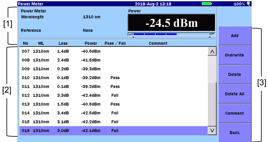
Figure 9.2-1 Loss Table Screen (Power Meter)
