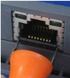
4. Keeping the tool STRAIGHT firmly pull the insert out from the socket.
