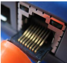
5. Using fingers replace a new insert STRAIGHT into the socket and secure in place by firmly pushing it home.
