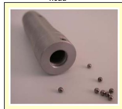
Fig. 4 – Detail of Aluminium armour head
