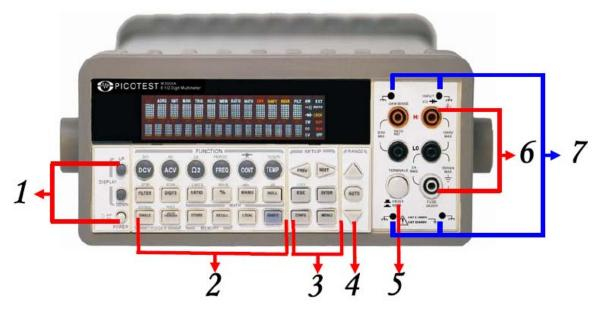
There are different buttons and terminals on the front panel. They are divided into the following groups: (DISPLAY & POWER), (FUNCTION, MATH, TRIGGER, MEMORY, SETUP, RANGE, INPUT TERMINALS), and (FILTER, DIGITS, LOCAL, and SHIFT) as shown in the previous figure
