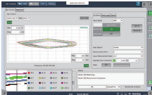
Example of Eye Contour Measurement at Input of Small 50 mVp-p Signal
