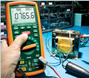
Measure the insulation resistance of transformer windings
