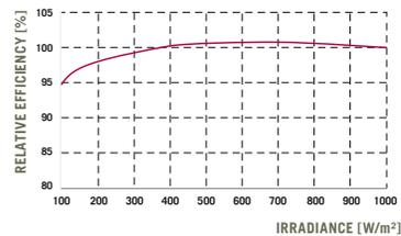
The typical change in module efficiency at an irradiance of 200 W/m<sup>2</sup> in relation to 1000 W/m<sup>2</sup> (both at 25 °C and AM 1.5 G spectrum) is -2 % (relative).
