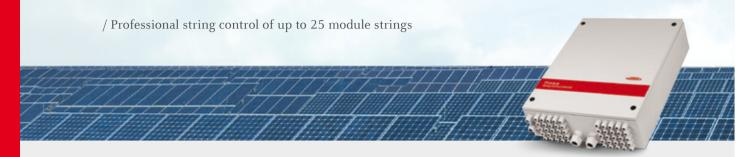
/ The Fronius String Control 250/25 and Fronius String Control 250/25 DCD DF can be used to monitor and bundle up to 25 module strings at a current carrying capacity of 250 A max. Fitting fuses in the fuse holder could not be easier. Continuous comparison of string currents reliably and quickly detects even the smallest fault occurring anywhere in the system.
