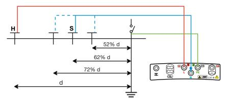
The 3 measurement results must be the same to within a few percent. If this is the case, the measurement is valid. If not, it is because the S rod is in the zone of influence of the earth electrode.
