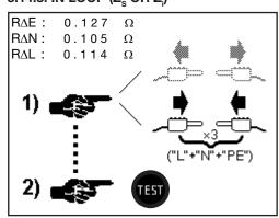
The current values of the compensations are displayed at top right. If the values are zero, no compensation has been determined.
