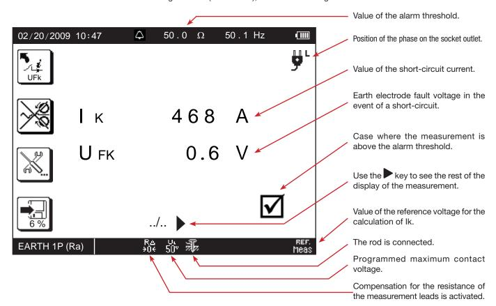
$U_{Fk}$  is calculated only in earth measurement on live circuit with a high current (TRIP mode).  $U_{Fk} = Ik \times Z_A$ .
