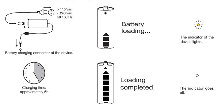
After prolonged storage, the battery may be fully discharged. In this case, the first charge may take longer and the indicator on the device flashes for the first few minutes.
