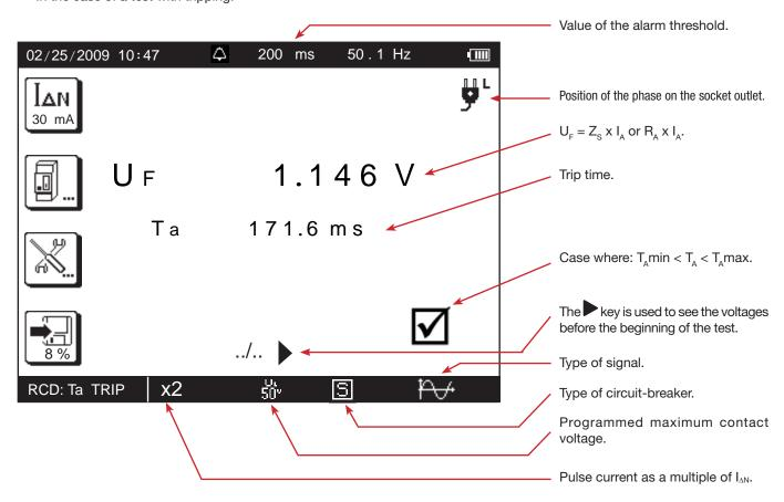
In the case of a non-tripping test:
