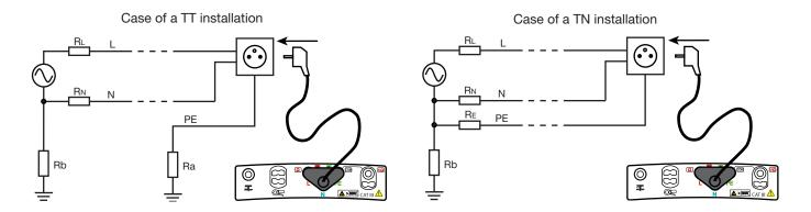
**Note:** in trip mode, it is not necessary to connect the N terminal.
