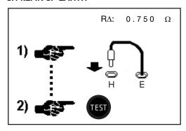
The current value of the compensation is displayed at top right. A value of zero indicates that no compensation has been determined.
