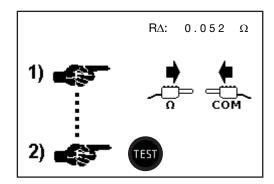
The current value of the compensation is displayed at top right. A value of zero indicates that no compensation has been determined.
