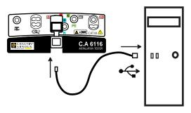
When the device is in communication with a PC, it does nothing else and its keys are inactive. It then displays the following message:
