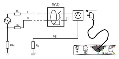
If possible, first disconnect all loads from the network on which you test the RCD. This prevents interference with the test by any leakage currents due to these loads.
