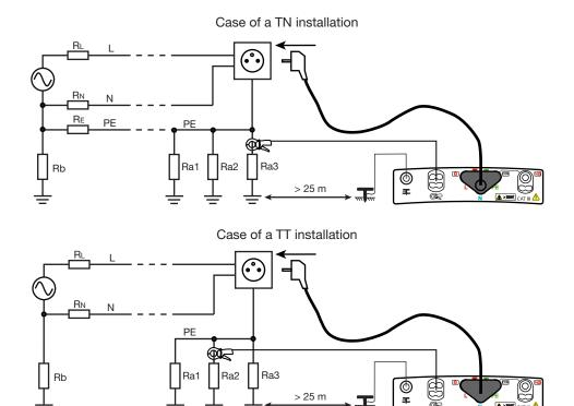
For greater accuracy, the measurement is made with a high current (TRIP mode). To avoid tripping out the circuit-breaker that protects the installation, you can short-circuit the circuit-breaker during the measurement, as follows:
