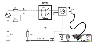
For a more accurate measurement of the fault voltage, plant the auxiliary rod at a distance of more than 25 metres from the earth electrode and connect it to the  $(R_A S_{EL})$  terminal of the device. The  $(R_A S_{EL})$  symbol is then displayed.
