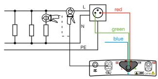
In the case of a three-phase network balanced in voltage and in current, connect the measuring cable terminated by 3 leads to the device and to two of the three voltages  $U_{12}$ ,  $U_{23}$  or  $U_{31}$  using the red and green leads. Then connect the clamp to measure the current on the opposite phase  $I_3$  (for  $U_{12}$ ),  $I_1$  (for  $U_{23}$ ) or  $I_2$  (for  $U_{31}$ ).
