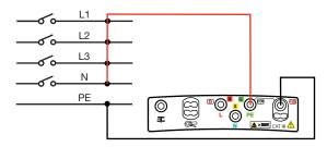
If the insulation is not sufficient, you must then make the measurement between each of the pairs to locate the fault. It is for this reason possible to index the recorded value with one of the following values:
