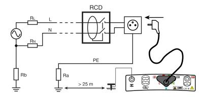
To make a more accurate measurement of the fault voltage, plant the auxiliary rod at a distance of more than 25 metres from the earth electrode and connect it to the  $(R_A S_{EL})$  terminal of the device. The  $(R_A S_{EL})$  symbol is then displayed.
