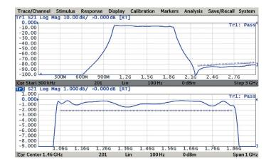
Limit testing is a function of automatic pass/fail judgment for the trace of the measurement results. The judgment is based on the comparison of the trace to the limit line set by the user and can consist of one or several segments.
