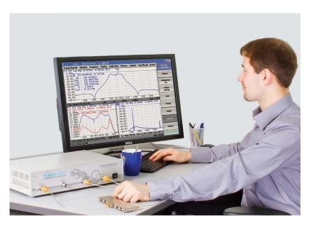
The Planar 808/1 VNA is an S-parameter vector network analyzer designed for operation with an external PC. It connects to any Windows-based computer via USB and delivers accurate testing and measurement through a platform that can keep up with constant advancements as well as be remotely accessed.
