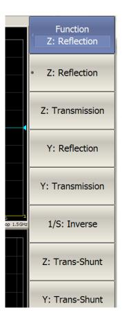
The function allows conversion of the measured S-parameters to the following parameters: reflection impedance and admittance, transmission impedance and admittance, and inverse S-parameters.
