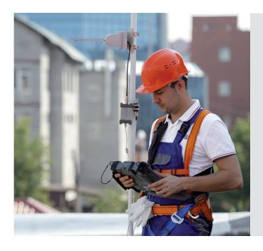
Planar R140 is a PC-driven vector reflectometer that operates in the frequency range from 85 MHz to 14 GHz. It is designed for use in the process of development, production, and field testing of various electronic devices in multiple environments, including operation as a component of an automated measurement system.
