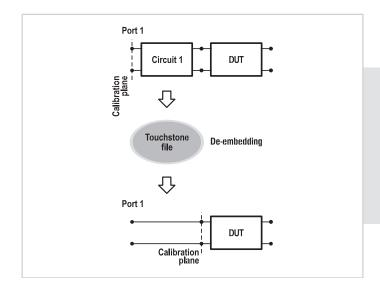
The function allows to mathematically exclude from the measurement result the effect of the fixture circuit connected between the calibration plane and the DUT. This circuit should be described by an S-parameter matrix in a Touchstone file.
