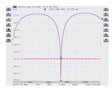
The return loss function measures the power lost in the reflection of the transmission. Planar R140 has a high accuracy and can measure return loss up to 35 dB in frequencies up to 4.8 GHz, and up to 25 dB in the frequency range 4.8 GHz to 14 GHz, which is a specification typical of benchtop instrumentation.
