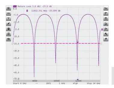
Testing in the frequency range 4.8 GHz to 14 GHz, the return loss is shown at 25 dB
