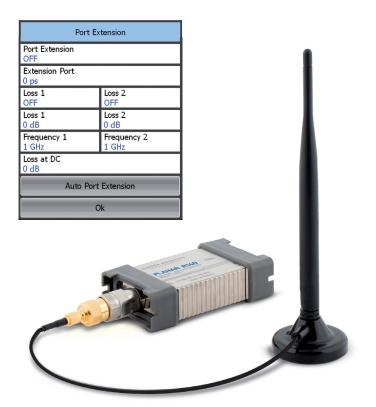
Port Extension is a feature that allows for moving the calibration reference plane of the port by specifying the electrical delay to the new reference plane position. Additionally, it is possible to account for loss in the extended port.
