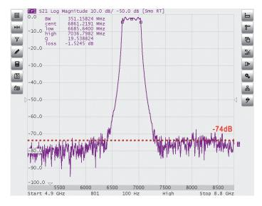
Typical dynamic range of measurement  $|S_{21}|$  using two reflectometers is 74 dB in the frequency range 4.8 GHz - 14 GHz (100 Hz IF bandwidth).
