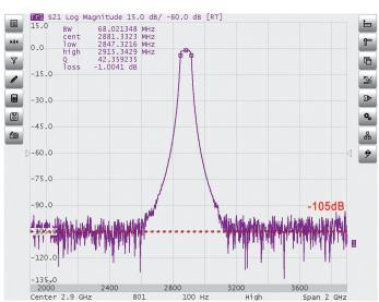
Typical dynamic range of measurement  $|S_{21}|$  using two reflectometers is 105 dB in the frequency range 85 MHz - 4.8 GHz (100 Hz IF bandwidth)
