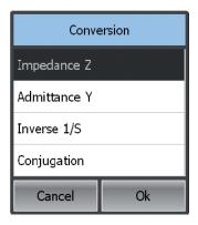
The function allows conversion of the measured S-parameters to the following parameters: reflection impedance and admittance, inverse S-parameters and conjugation.
