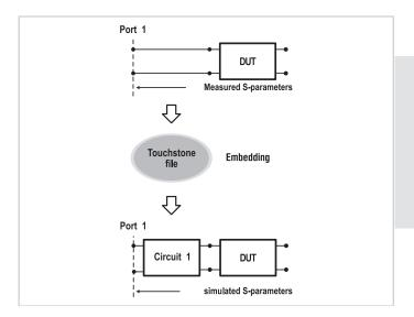
This function allows the user to mathematically simulate the DUT parameters after virtual integration of a fixture circuit between the calibration plane and the DUT. This circuit can be described by an S-parameter matrix in a Touchstone file.
