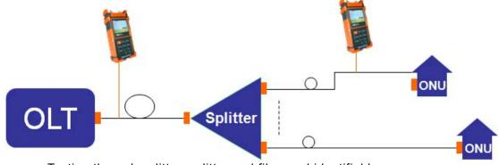
· Testing through splitter, splitter and fiber end identifiable
