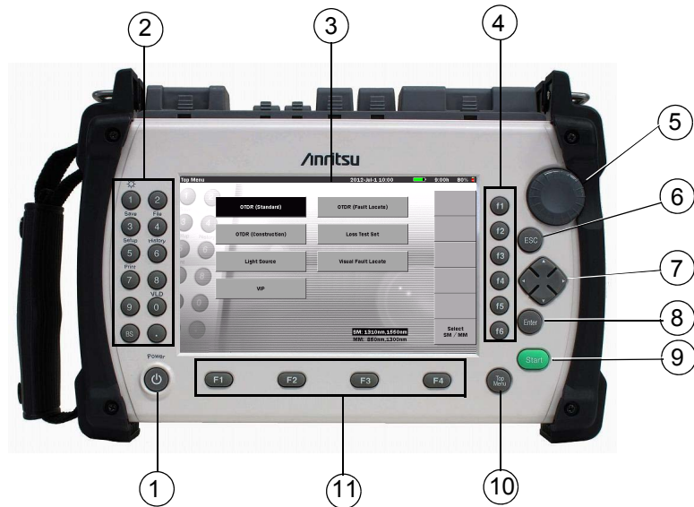
Figure 2-1: MT9083 Series – Front Panel
