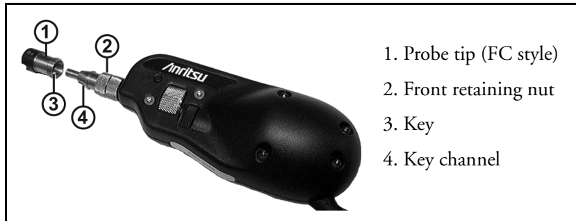
Figure 11-4: Attaching a Probe Tip
