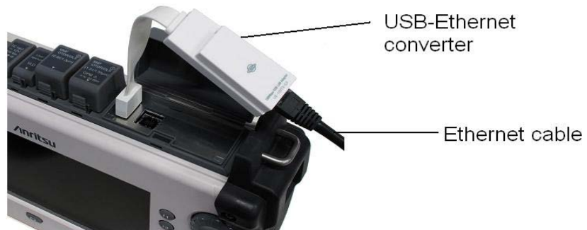
Figure 14-2: Ethernet Cable Connection
