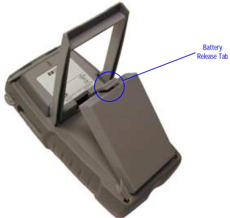
Flip out the stand at the back of the unit and press the battery release tab to release the top edge of the battery pack. Rotate the battery pack towards the bottom of the unit and then pull the battery up and back to remove it from the back of the unit.
