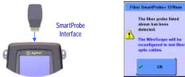
The key to providing this capability is that the SmartProbe interface port warns the operator if there is a potential invalid configuration before testing starts.
