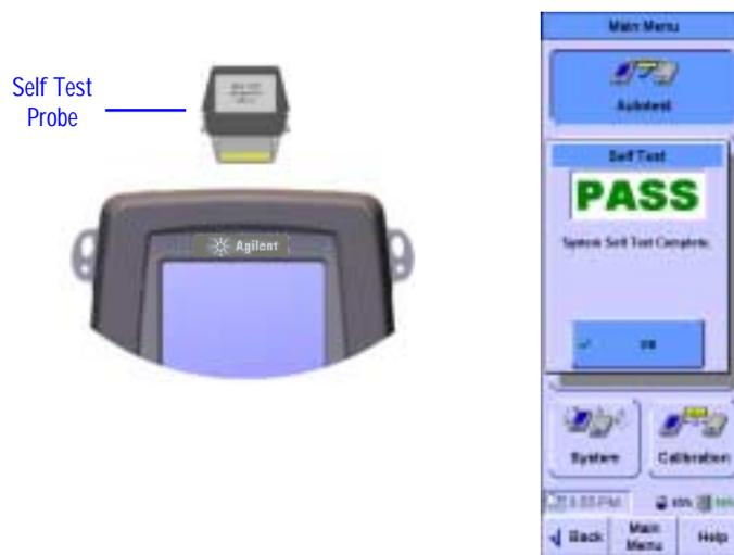
A passing self test indicates that the baseline calibration data for the WireScope 350 is still valid. If the self test fails, the WireScope 350 requires a new baseline calibration or repair. Please contact WireScope technical support if the self test fails.
