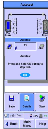
If you have not connected to the DualRemote 350, a “Searching For Remote” dialog box will come up until you connect the DualRemote 350. If the DualRemote 350 is connected to the other end of the cabling run, the progress indication dialog will come up. A bar graph will update as the test progresses. To stop the test before it is complete, press **OK**.
