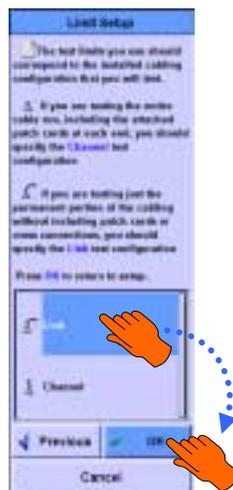
The second step is selecting the test configuration (such as Link or Channel ), since each test configuration requires a slightly different set of limits to account for the number of connections included. Press **OK** or **OK** to finish making the limit setting and return to the Autotest Settings screen.
