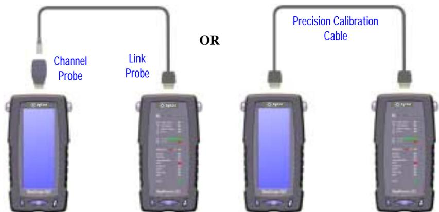
If you are testing link configurations to Category 6 / Class E or higher, Agilent Technologies recommends that you use the precision calibration cable, as this produces the most accurate calibration.
