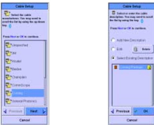
The first Cable Setup configuration screen prompts you to specify the manufacturer of the cable that you will be testing. If you do not know the manufacturer, select “Unspecified”. Use the **+** key if you need to scroll the list of manufacturers. In the example above, Corning is selected.
