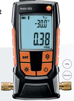
The testo 552 is a digital vacuum measuring instrument for the evacuation of refrigeration systems and heat pumps. It measures even the smallest absolute pressures and provides highly precise information on the status of the dehumidification of a system (removal of foreign substances, incl. oils or foreign gases).
