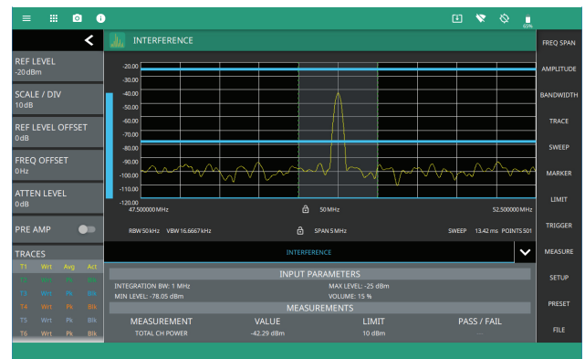
Interference Finder Option 0024 Provides Fast Audio Tone Response to Changing Interference Levels
