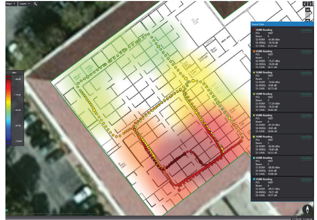
Typical Result Screen for Indoor Coverage Mapping
