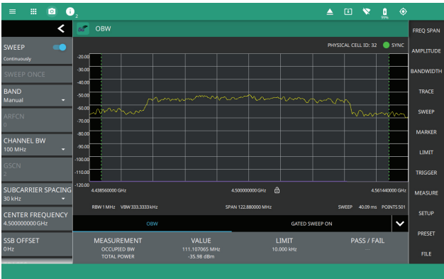
Automated Occupied Bandwidth Measurement Result for a 100 MHz 5G NR Radio
