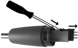
An illustration showing a screwdriver with a black handle and silver shaft. The tip of the screwdriver is inserted into a slot on the side of a cylindrical probe. An arrow points to the right, indicating the direction of force applied to pry the probe's tip away from the thermocouple head. The thermocouple head is shown as a separate component with two electrical leads.
