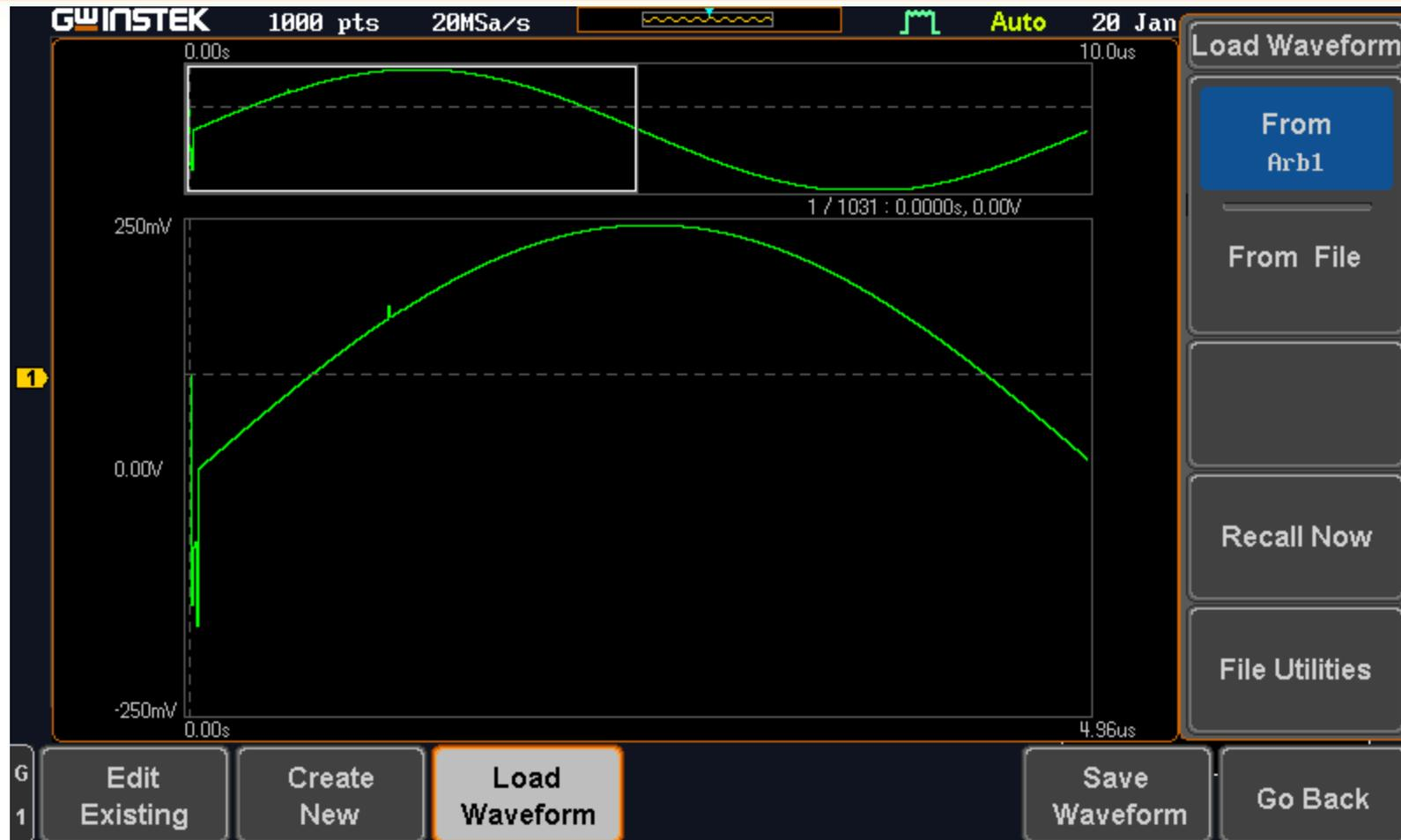
User is allow to load and create arbitrary waveform on the MDO-2000E series .
