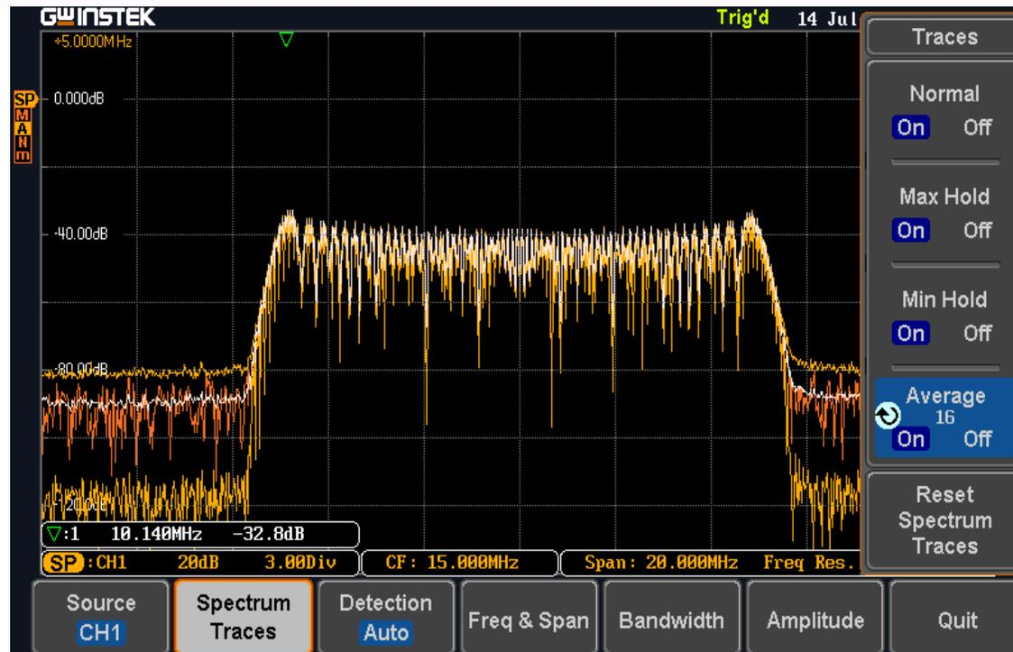
In order to allow users to experience genuine Spectrum Analyzer, MDO-2000E also includes Spectrum Trace Type settings (Normal, Max-hold, Min-hold, and Average). Users can freely simultaneously select various Spectrum Traces.
