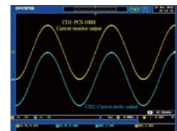
PCS-1000I vs. Current Probe for Measurement
