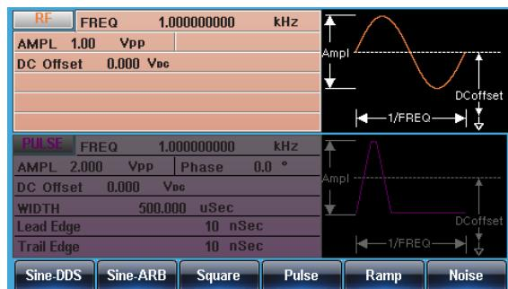
2. Press F5 (Ramp) to create a ramp waveform.
