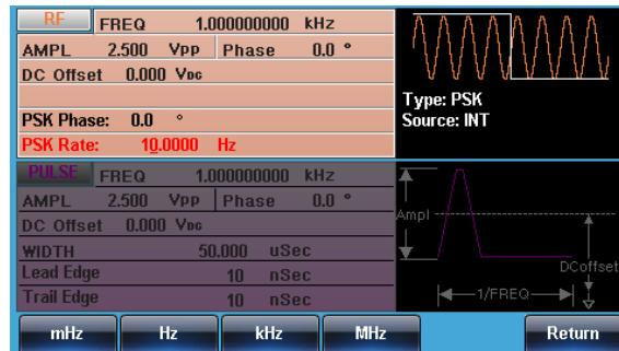
5. Use the arrow keys and scroll wheel or number pad to enter the PSK rate.
