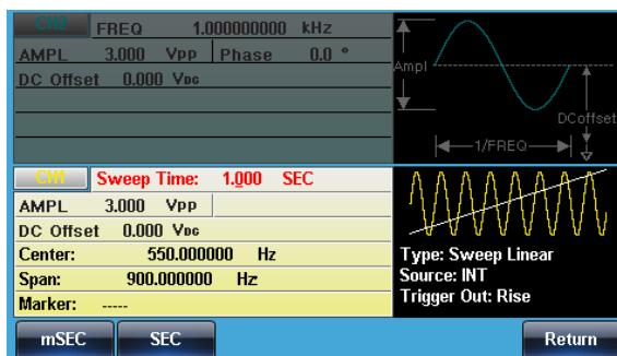
4. Use the selector keys and scroll wheel or number pad to enter the Sweep time.
