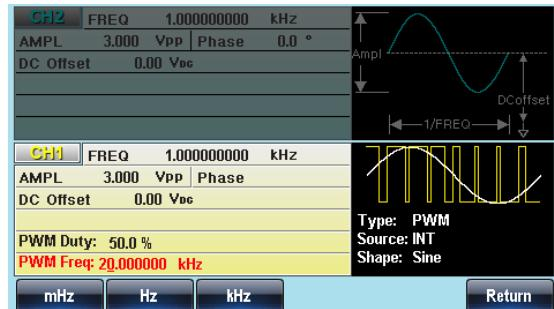
5. Use the selector keys and scroll wheel or number pad to enter the PWM frequency.
