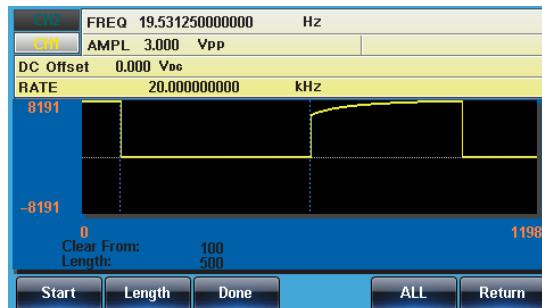
The result after the whole waveform is deleted:
