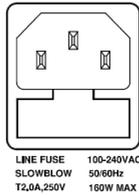
The AC input accepts 100 to 240  $\pm 10\%$  VAC. The frequency is 50Hz/60Hz. Fuse: 2A slow-blow type See page 138 for details.
