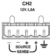
A total of 5 ports: 1 positive output terminal, 1 negative output terminal, a Sense+ terminal, a Sense- terminal and a ground terminal. Refer to the printed label under the terminals for the specific order of the terminals.
