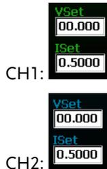
**Parameter Settings Display** Displays the relevant parameter settings. For details on setting parameters, see page 20. The following figure shows the basic power source for both channels (V AND I)
