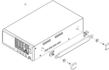
2. Remove the six screws on both sides and the four screws on the rear.
