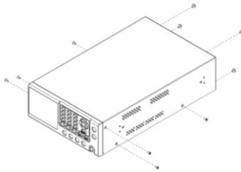
3. Open the cover. Find the location indicated by the arrow in the figure shown below and then replace the battery with a new one.
