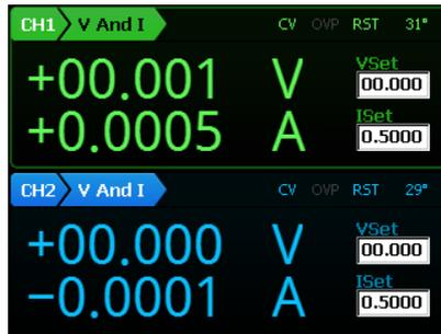
**Voltmeter Indicators** Displays the output voltage with up to 5 digits of resolution. The default units are Volts (V).
