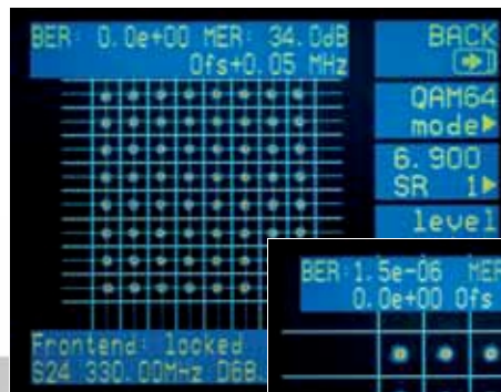
Constellation diagram of a QAM64 signal
