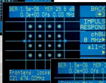
Constellation diagram of an OFDM signal (16QAM)
