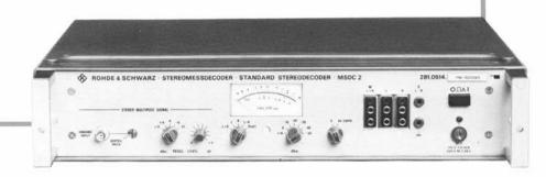
The Precision Stereodecoder MSDC 2 is used to measure and monitor stereo multiplex signals. Its performance far exceeds the requirements set by ARD in all significant points. Thus the MSDC 2 can be employed as a reference standard in the development and production of stereo coders and decoders, as well as in transmitter networks to ensure high transmission quality.
