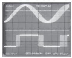
When signals are displayed in the envelope mode, the influence of jitter effects, amplitude changes and aberrations can be demonstrated significantly. The scope builds the envelope curve by storing the minimum and maximum values over a number of consecutive sampling periods.
