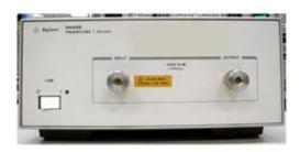
The Agilent 8449B microwave preamplifier is a high-gain, low-noise preamplifier that provides additional sensitivity for any RF/microwave spectrum analyzer for detection and analysis of very low signals. The improved sensitivity can dramatically reduce measurement time.
