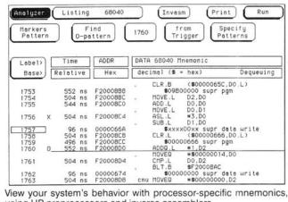
View your system's behavior with processor-specific mnemonics, using HP preprocessors and inverse assemblers.
