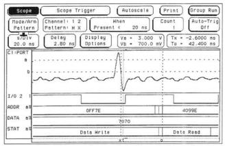
Pinpoint design errors and show their effects by integrating timecorrelated scope and timing waveforms.
