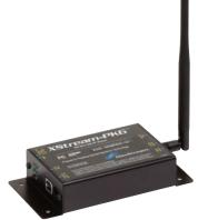
The 2635A-RF900 and 2635A-RF900USB are RF (radio frequency) modems for wireless operation of Hydra Series data acquisition instruments. They provide a wireless link between a Fluke Hydra Series unit and a computer running Hydra application software.
