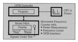
Frequency domain analysis may be accurately performed with a microwave frequency counter in a simple setup.
