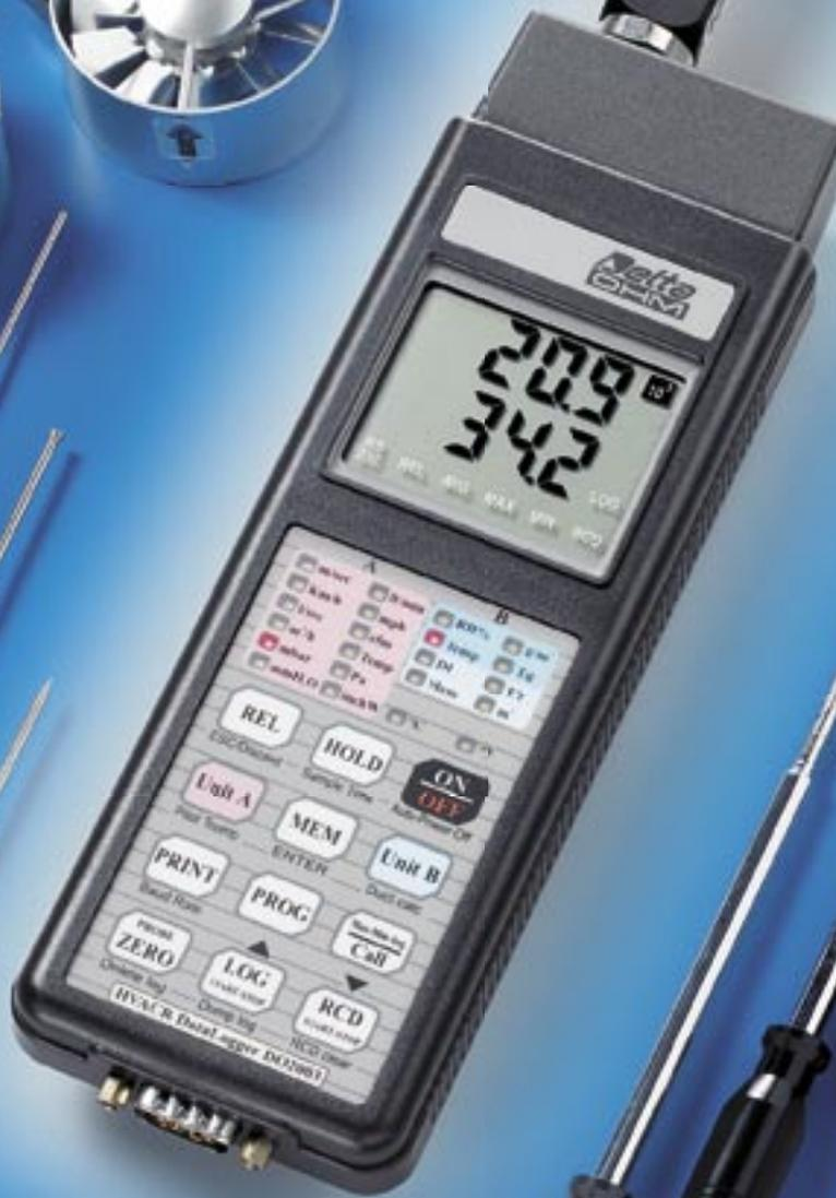
**VELOCITÀ E PORTATA DELL'ARIA - TEMPERATURA - TEMPERATURA/UMIDITÀ RELATIVA - PRESSIONE**
