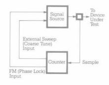
Only three interconnections are required to coarse tune and phase-lock an electrically-tunable source:
