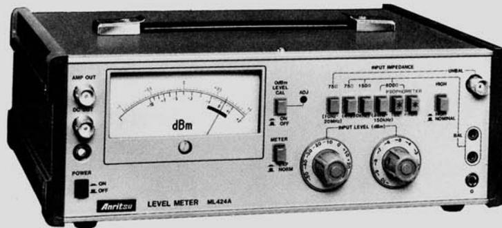
The ML424A/B is a compactly designed level meter of high level measuring accuracy with calibrated signals internally provided. It is also capable of measuring noise levels (in conformity with the CCITT Recommendations) with the necessary psophometer option.
