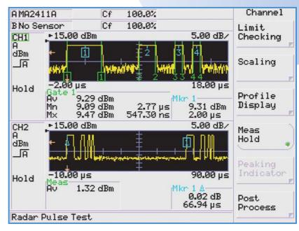
Examine the pulses in detail and capture the entire pulse train.
