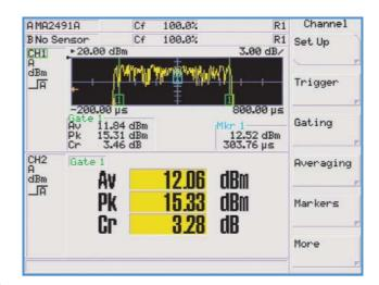
The user can choose between several measurements performed within the gate. Average, peak, crest, max and min are available as selections for the output.
