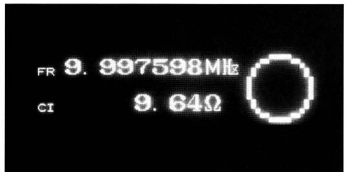
▲ GO/NO-GO testing of a crystal oscillator
