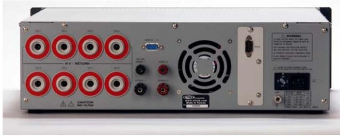
*With its built-in HV Scanner, the V5 can automatically conduct both Hipot and IR tests on up to 8 different points. Rear panel terminals provide convenient access for Ground Bond testing, while PLC, RS232 and available GPIB interface connectors allow for easy systems integration.*
