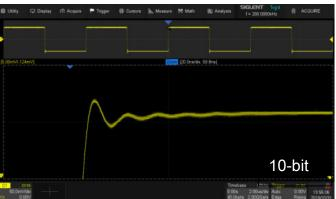
10-bit mode combined with Zoom shows you more details and less noise on the waveform.
