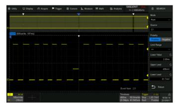
The SDS2000X Plus can find events within a record and history based on user specified trigger conditions. Navigate browses through Events flagged by the Search, plays back history frames or continuously moves the delay position on long records (useful in zoom view).
