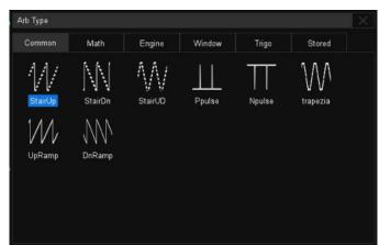
The built-in DDS waveform generator can output waveforms with up to 50 MHz frequency and ±3 V amplitude. Six basic waveforms together with multiple types of predefined waveforms and as user defined arbitrary waveforms are supported.
