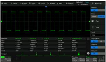
Measurements can be performed within a specified gate period. Measurements on Math, Reference and History frames are supported.
