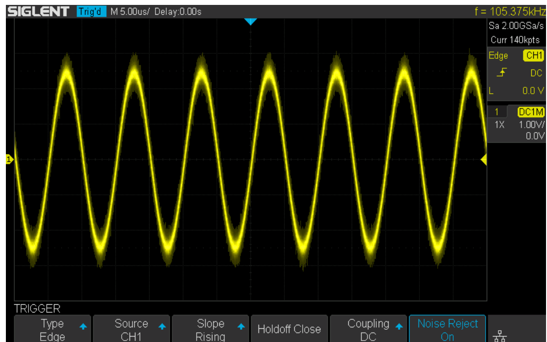
Figure 23 Noise Rejection enabled
