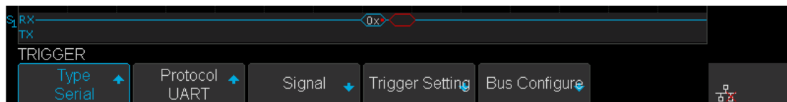
Figure 52 UART Decode Bus Display
