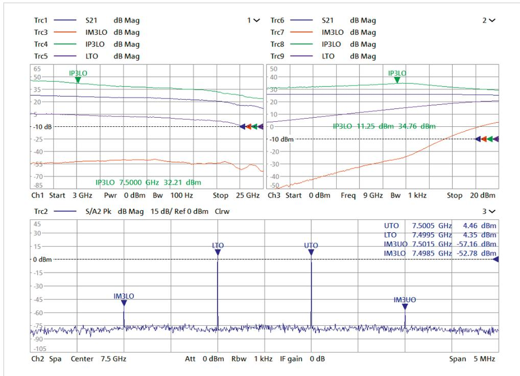
Comprehensive amplifier characterization, including intermodulation products (IP), IP versus frequency, spectral measurements and other quantities
