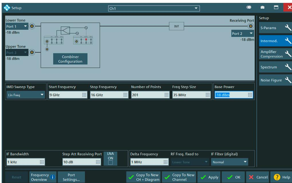
Configuration GUI for an amplifier intermodulation test
