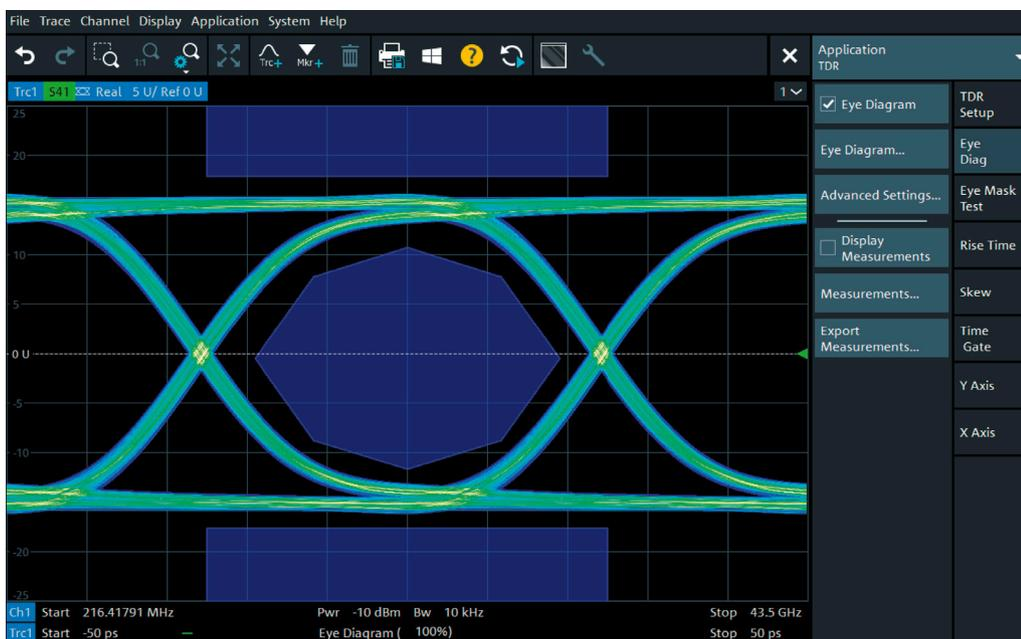
The R&S®ZNA-K20 option offers versatile signal integrity measurements, e.g. eye diagrams with a mask to verify compliance with relevant requirements. It can also be used to determine the transmission characteristics of signals with jitter or noise.
