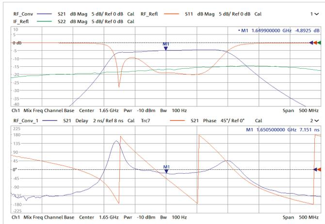
calculates the group delay and the relative phase. The frequency drift and frequency modulation of the DUT's internal LO do not affect the measurement accuracy as long as the frequency deviation lies within the analyzer's IF bandwidth used for the measurement.
