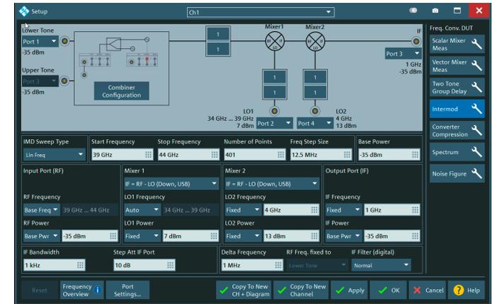
All-in-one dialog for intermodulation measurement on a double converting receiver
