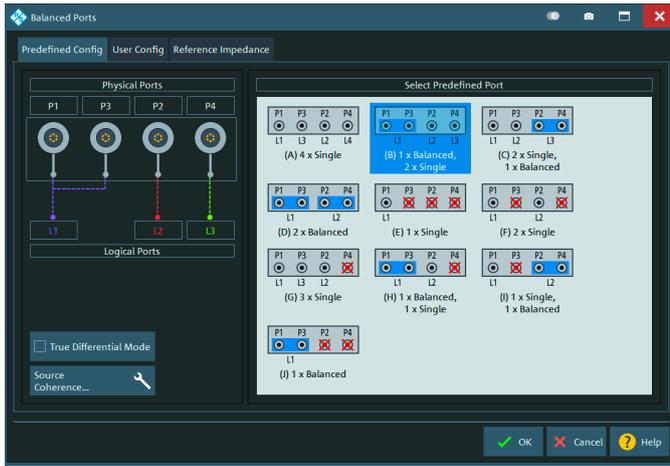
Balanced structures as well as used and unused ports are defined at a keystroke. Predefined topologies are completed with a tab offering free user configurations.
