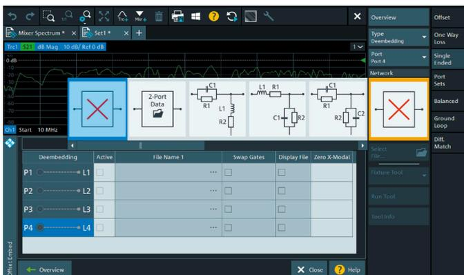
The R&S®ZNA comes with a choice of predefined matching networks whose values can be edited. If values are changed, the R&S®ZNA will immediately recalculate the network and embed the DUT in the new network in real time.
