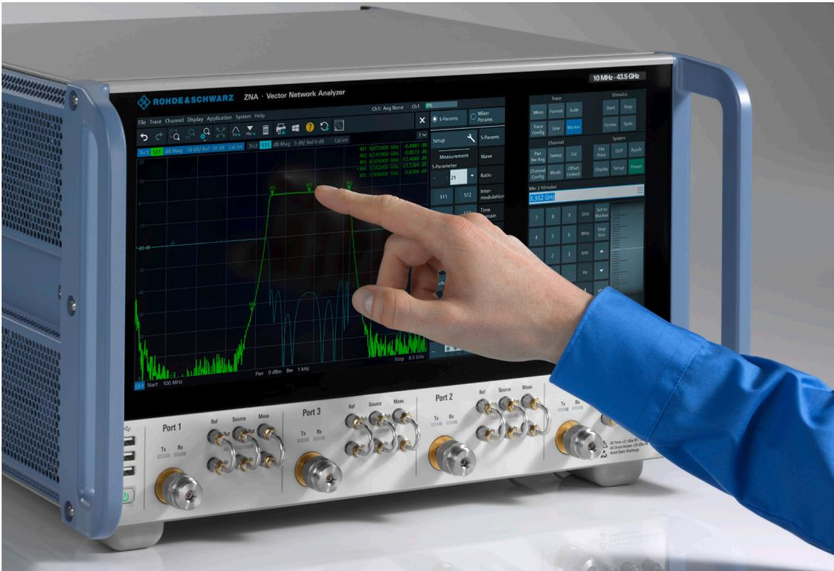
The analyzer's DUT-centric operating concept makes it possible to achieve the desired setup at an unrivaled speed. Users can control sophisticated measurements at a glance with dedicated dialogs that show the setup schematics and all of the essential test parameters.
