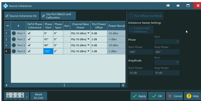
GUI for entering dedicated port specific values for phase and power. In automatic true differential measurement mode, users can enter parameters for phase and magnitude imbalance sweeps.
