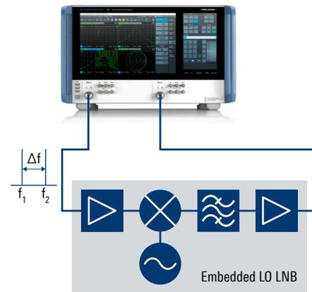
Example result screen of embedded LO converter testing: conversion gain, group delay, noise figure, compression, intermodulation
