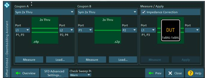
For in-fixture and PCB tests Rohde & Schwarz offers advanced coupon based deembedding options, supported by a smart configuration wizard.
