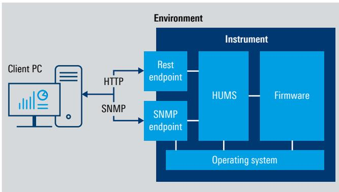
HUMS is available on the R&S®ZNA with the R&S®ZNA-K980 software option. HUMS opens the SNMP agent and a REST service with HTTP endpoints, which allows the HUMS data to be retrieved.
