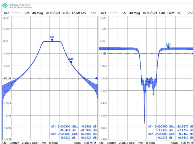
The R&S®ZNA-K50(P) option requires installation of the the VNA tool from the Swiss metrology authority METAS. This option enables operators to use the VNA tool as an additional means of individual uncertainty evaluation.
