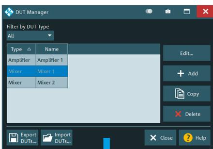
Based on the DUT type, the user is prompted to select and configure the desired measurements in a step-by-step process. The required channels and traces, e.g. for measuring LO feedthrough, are automatically created.
