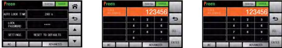
In order to prevent the operator from changing the set parameters by mistake, the new Screen Lock Password function is added on AFV-P series, so that the operator can only perform the output of the device, and only authorized personnel has the password to unlock the screen and edit parameters.
