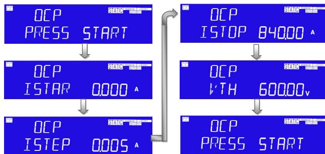
**ISTAR:** setting the start current point, the Left 5 digit monitor display the “OCP”, the right upper 5 digit monitor display the “ISTAR”, and right lower monitor display setting value, the unit is “A”. The range is 0.001A to the full scale of the CC mode specification. The setting is by rotating the setting knob.
