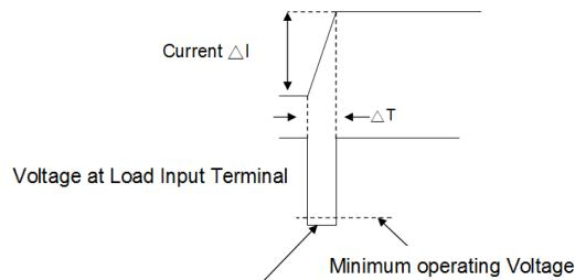
When the Voltage drops under minimum operating voltage, the electronic load may generate unstable oscillation
