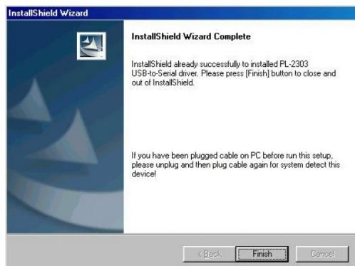
2. After the installation, connect the PEL-5000C series and PC with USB. Then select the item USB to Serial Port (COM3), set the BAUD-RATE and Flow control to 115200bps and Hardware to control PEL-5000C series with COM3.
