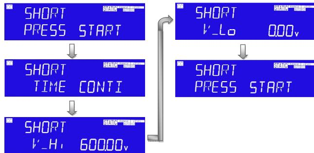
Set the short test time, the LCD display show "SHORT" on left 5 Digits LCD display, shows "TIME" on middle 5 digits LCD display, right 5 digit LCD display "CONTI", the unit is "ms".
