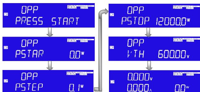
PSTAR: setting the start power, the LCD display shows "OPP" on left 5 digit LCD display, middle 5 digit LCD display "PSTAR", right 5 digit LCD display setting value, the unit is "W", the setting range is 0.00W to the full scale of the CP mode specification. The setting is by rotating the setting knob.
