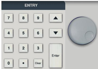
**Rotary Knob and ARROW Keys** The ROTARY knob and ARROW keys are used to increase or decrease the set values.
