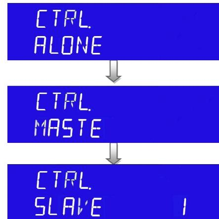
The following procedure should be followed before applying power on Master/Slave mains:
