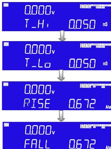
Press DYN setting key, LED will ON setting level High Period, Middle 5 digit LCD display will show "T-Hi" Right 5 digit LCD display will show setting value, the unit is "ms", The T-Hi set range from 0.010 ms to 9999 ms step 0.001ms by rotating the setting knob.
