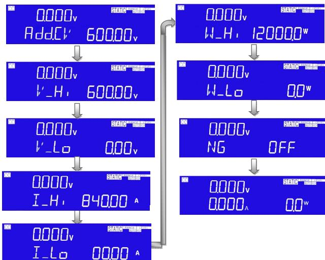
Setting CC+CV or CP+CV upper limit voltage, Middle 5 digit LCD display "Add.CV", right 5 digit LCD display the unit is "V", The Add.CV set range from 0.00 V to 600.00V step 0.01V by rotating the Setting knob.
