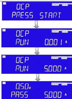
8. The UUT's output voltage drop-out lower than the threshold voltage(V-th setting), and the OCP trip point is between I\_Hi and I\_Lo limitation, then middle 5 digits LCD display will shows "PASS", otherwise shows "FAIL".
