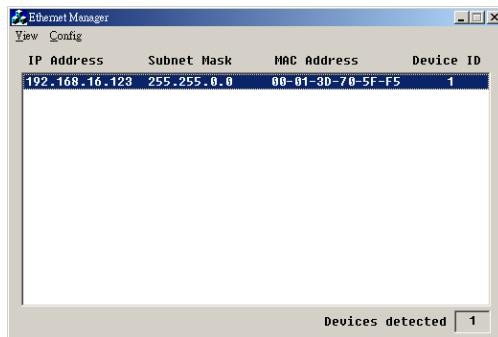
3. It will be shown the installation which has been searched on the screen , click it and select the Set IP Address bellows Config :
