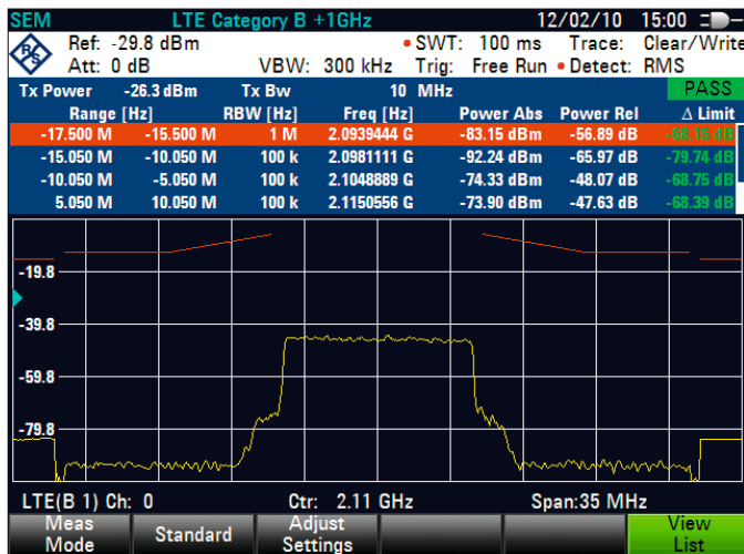
Spectrum emission mask measurement on an LTE signal.
