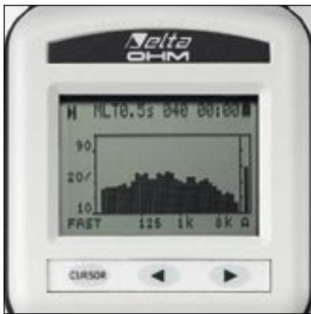
Dynamic range measurement for wide band and constant percentile band channels : 20÷140dBA on two ranges of 110dB (20÷130dBA and 30÷140dBA).
