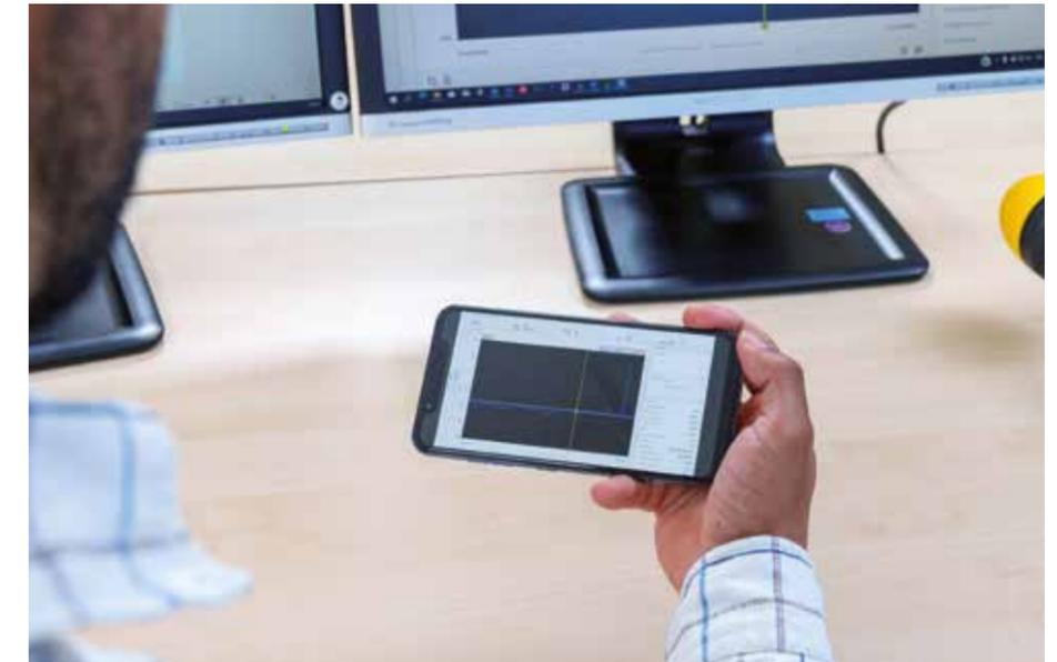
↑ The WiFi / Bluetooth interface enables remote control of the FieldMan via the optional smartphone app. In this way, you can create photos and videos that can be added to the measurement data.
