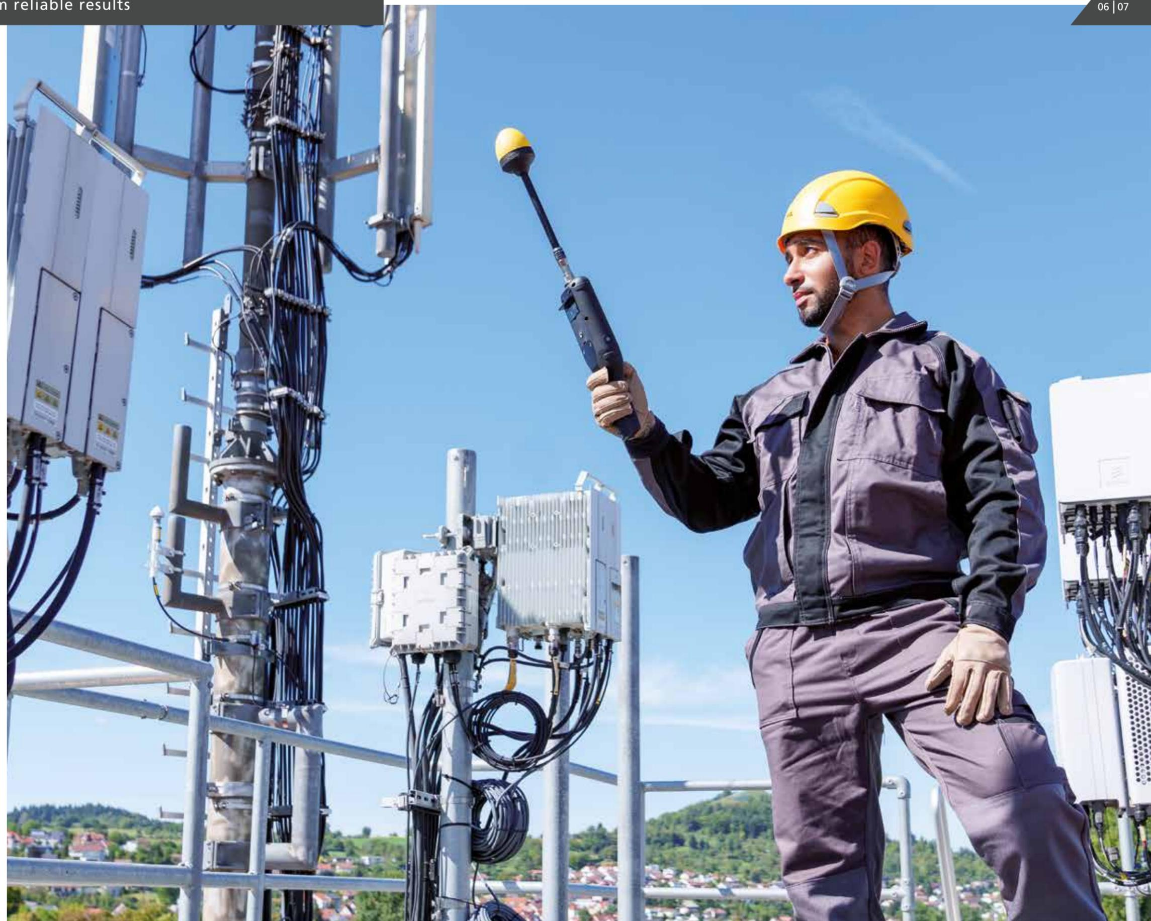
→ The FieldMan also shows its strengths during everyday use with its various storage and readout facilities. A Micro SD card makes it super easy to personalize. The optional WiFi / Bluetooth interface enables remote control using the smartphone app.
