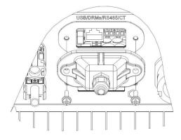
**Step2** Unlock the waterproof cable gland, remove the stopper in the waterproof connector;
