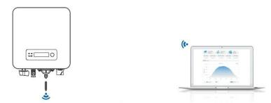
The operation information (generated energy, alert, operation status) of the inverter can be transferred to PC or uploaded to the server via Wi-Fi. You can register on the website.
