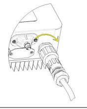
Removing the AC connector Pull out the AC connector by rotating the knob
