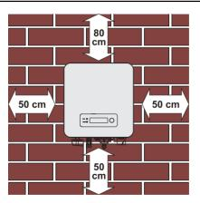
clearance for single 1.1K~3.3KTL-G3 Inverter Installation of multiple 1.1K~3.3KTL-G3 inverter
