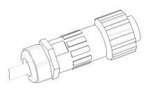
**Step 5** Connect the AC connector to the output wiring connector of inverter, rotate the AC connector clockwise until the fastener reaches its designated position, as shown below.
