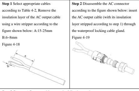
Step 3 Connect AC output cable as per the following requirements:
