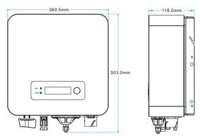
Figure 2-3 Front view and left view dimensions of 2700TL-G3, 3000TL-G3 and 3300TL-G3
