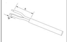
**Step2** Disassemble the AC connector according to the figure shown below: insert the AC output cable (with its insulation layer stripped according to step 1) through the waterproof locking cable gland;
