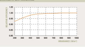
The typical relative change in module efficiency at an irradiance of 200 W/m² in relation to 1000 W/m² (both at 25  $^{\circ}C$  and AM 1.5 spectrum) is -7%.
