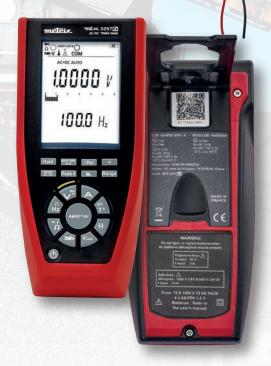
The MTX 3297 is equipped with 4 qualified lithium batteries (plastic protective film for transport as per the regulations) for a battery life of 350 hours in the field.
