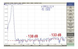
Typical dynamic range of 125 dB is achieved from 300 kHz through the top of the frequency range (at 10 Hz IF bandwidth). Seen here is the maximum dynamic range achieved when using IFBW 1 Hz and an output power level of 5 dBm.
