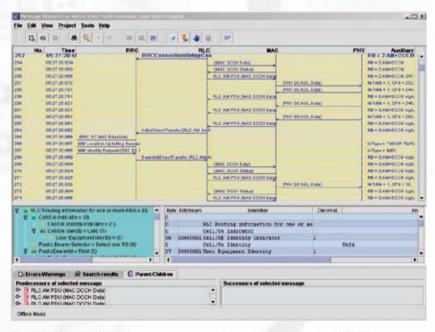
The R&S® CMU-Z46 WCDMA message analyzer and recorder option records all UTRAN protocol layers affected by communications between the R&S® CMU200 and the mobile phone. The top half of the screen shows a list of all recorded protocol layers. The individual layers can be selected and their contents analyzed in detail (bottom half of screen).
