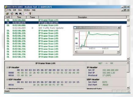
Recording of all exchanged IP data packets with time stamp and display of the data transmission rate achieved.
