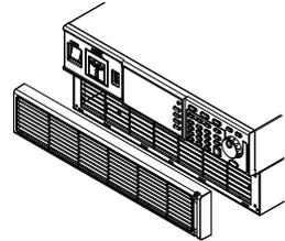
12. Replace the filter with a new one.
