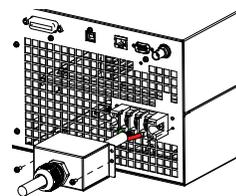
3. The AC power cords are perfectly connected with the AC input terminals.
