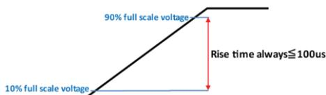
**Slope** The rising slew rate is constantly fixed in  $1.5\text{ V}/\mu\text{s}$  with varied rising time in accord with differed output voltage scale.
