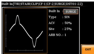
DST01-22 The DST01-22 waveform shape function simply adds a number Fourier series terms to create an arbitrary waveform.
