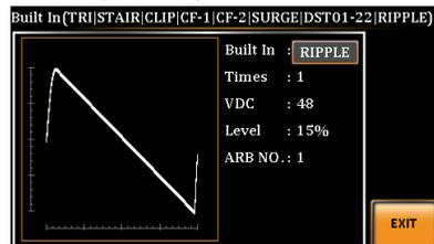
**DIP** (ASR-3400HF only) The DIP waveform refers to a transient reduction in RMS voltage, also known as Voltage Dip or “Drop In Point”. Refer to following for the suggested range.
