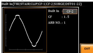
SURGE The surge waveform has a settable ACV base level, site size and site shape.
