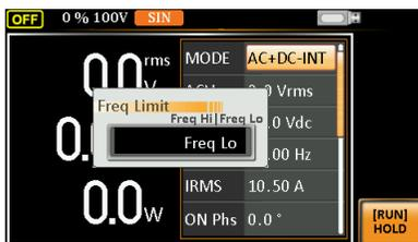
3. Set the frequency limit with the scroll wheel or with the F3 ~ F4 soft-keys. The MAX and MIN soft-keys set the frequency limit to the maximum and minimum, respectively.
