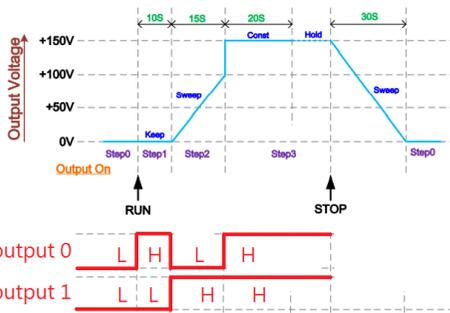
The example above shows how to generate a test procedure in DC-INT mode by each step.
