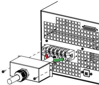
4. The output AC power wires are perfectly connected with the AC output terminals.
