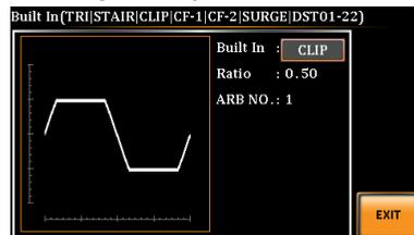
CF-1 Crest factor (CF-1) waveform. The crest factor is settable.
