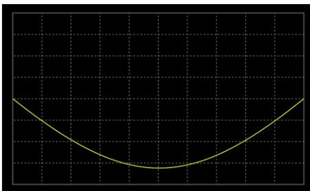
ARB 5 Sine wave, half-wave rectification (positive polarity)
