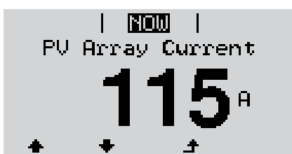
PV Array Current Current that is being supplied at present by the solar modules (Ampere)
