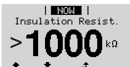
Insulation resistance of the photovoltaic system (kOhm) in the case of non-grounded solar modules
